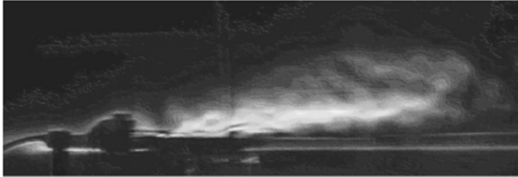
Fig. 6. Shadow photograph of the induced flow in measuring the velocity by the mathematical-pendulum method.
