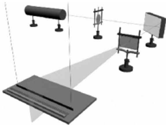
Fig. 3. Diagram of the setup for measurement of the induced-flow velocity.
